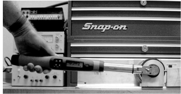
Fig. 1 Loosen to CAL, set 10% of F.S. to CHECK. Fig. 2 Bias wrench up against index
